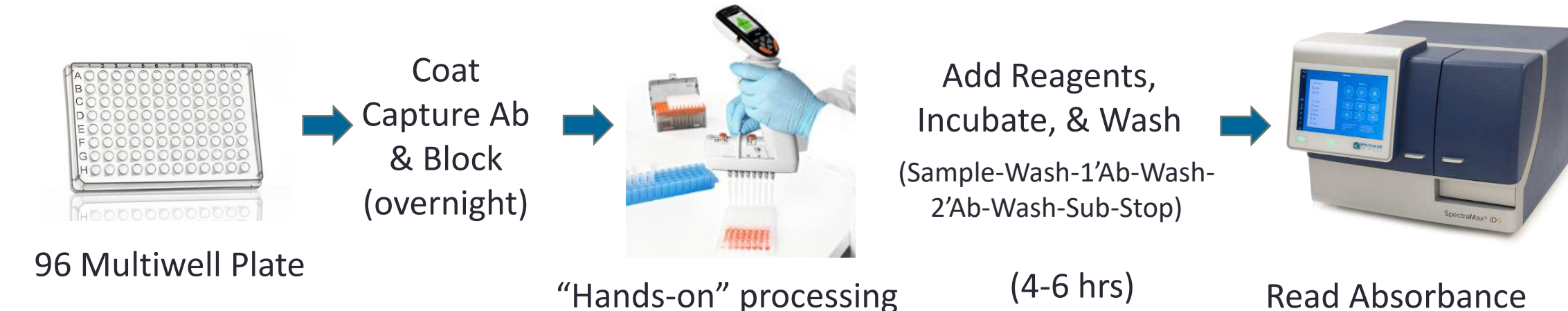
Figure 2. ELISA workflow for automated Pu-MA System and general protocol for complete 96-well plate ELISA.
