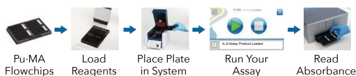
Figure 1. Schematic Pu·MA System assay workflow.
