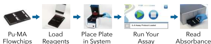
Figure 1. Schematic Pu·MA System assay workflow.
