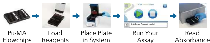
Figure 1. Schematic Pu·MA System assay workflow.
