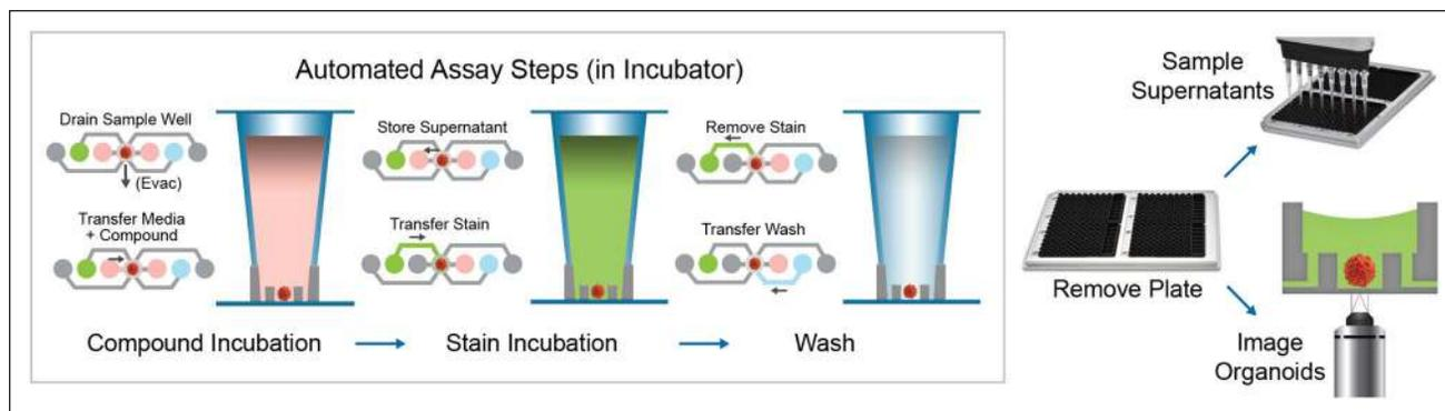
**Figure 3.** Fluid transfer steps presented for compound incubation, organoid staining, and stain removal by wash. Plates can be easily moved in and out of the system for downstream analysis. After a plate is removed from the Pu·MA System, supernatants can be removed for an enzyme-linked immunosorbent assay (ELISA) or other analysis. Microtissues can be imaged using an automated confocal imaging system or processed for other readouts.
